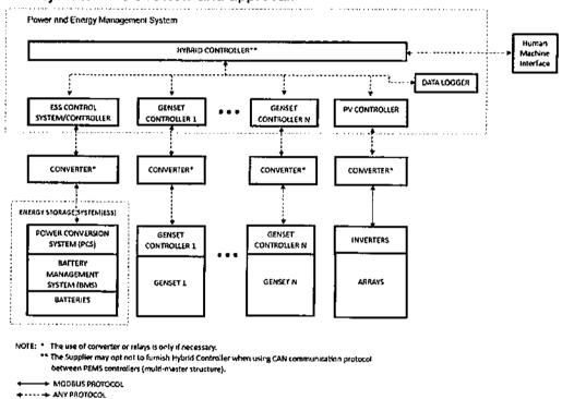
Figure 1: PEMS and Communication Diagram
